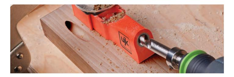
**Image 1** This shows a common thickness of 19mm. Pilot drill should just break through by 1-3mm.
