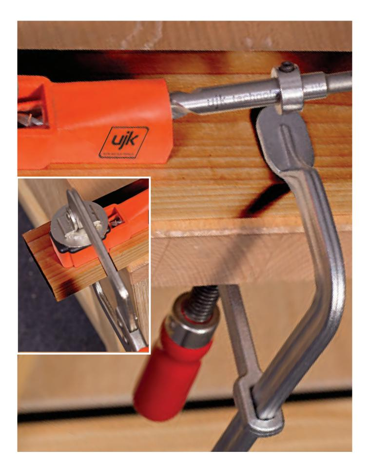
Image 8 Move the jig across using the same pencil line to position and repeat drilling. The number of pocket holes will depend on the material width.
