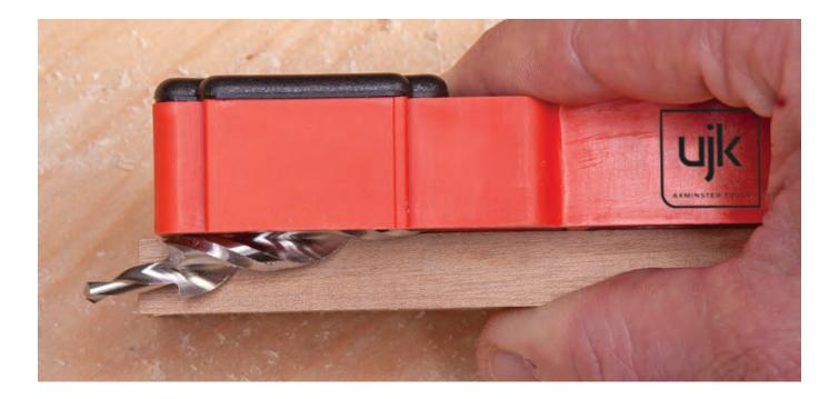
**Image 3** If using thicker material move the jig back and increase the drill depth.
