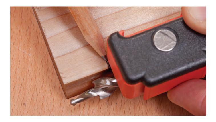
**Image 6** Clamp the guide to the timber and workbench. Use the marked line to position the jig and drill (at high speed) with the depth set drill.
