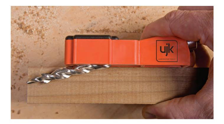
**Image 4** Lock the drill depth collar.
