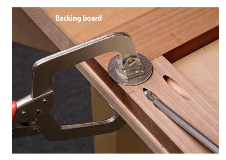
**Image 10** To assemble the joint the UJK Technology fence clamp is ideal as it has a large pad to help keep the two pieces flush with each other during assembly. Use UJK Technology pocket hole screws, please refer to chart. Use a 150mm long Torx 20 driver. Make sure you use the correct torque setting on the drill and ensure the screw is not over driven.
