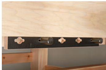
Side dogs ensure the work piece is perfect in the horizontal or vertical position
