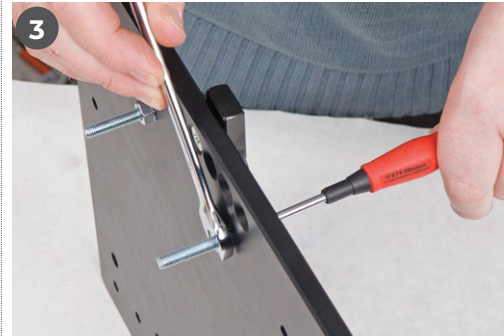
Tighten using a Phillips screwdriver and open ended spanner
