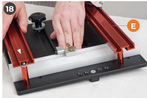
18 Line up the oval nuts in the height spacers (J) with the 'T' slots in the guide rails (E) and slide the guide rails on
