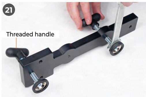
21 Holding the assembly (H) in place attach the threaded handles
