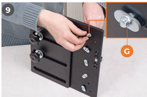
Put to hand the five Phillips screw with oval nut (G). Remove the oval nuts, slot the screws through the countersink holes in the base plate (C) and reattach the oval nuts, see illustration above.
