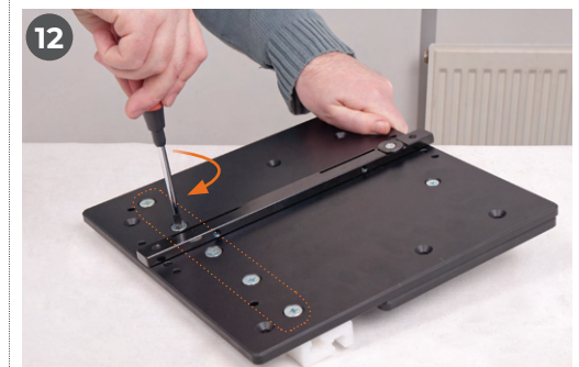
Turn the assembly over and tighten the five Phillips screws to secure the nylon sled fence in position
