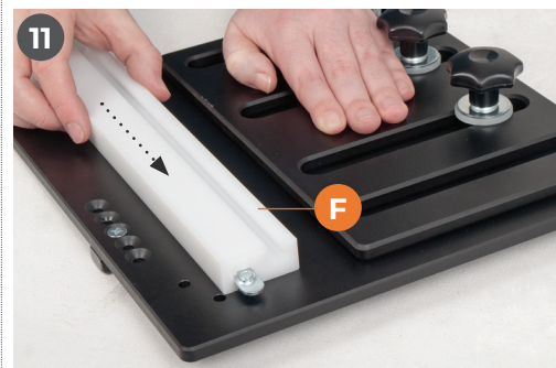
Locate the nylon sled fence (F), insert the first oval nut (G) into one of the machined 'T' slots in the nylon fence (F) and slide the fence on. Repeat the procedure for the remaining oval nuts until the nylon fence is in line with base plate (C) sides.
