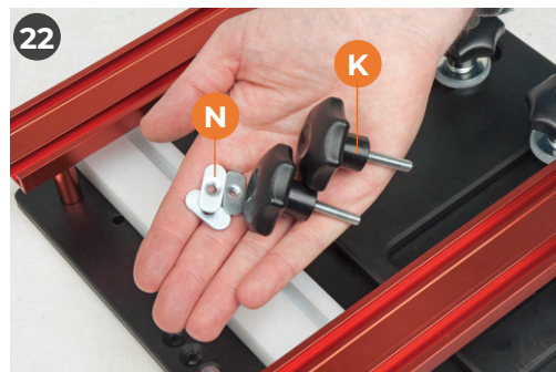
22 Put to hand three oval nuts (N) and the two threaded knobs (K)
