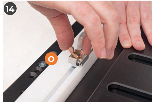
14 Manoeuvre the 'Adjustable Stop' (O) to the centre of assembly (F) and lightly tighten the butterfly nut
