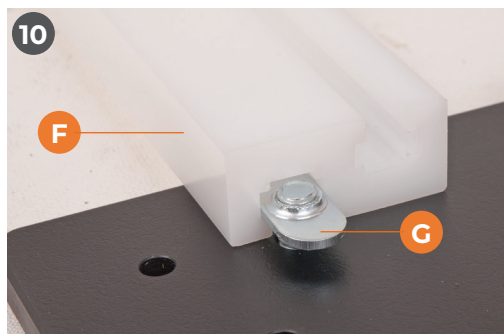
Locate the nylon sled fence (F), insert the first oval nut (G) into one of the machined 'T' slots in the nylon fence (F) and slide the fence on. Repeat the procedure for the remaining oval nuts until the nylon fence is in line with base plate (C) sides.
