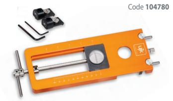
**4.** For greater precision a vernier scale with a micro adjuster (4) allows you to set the jig with an accuracy of 0.1mm. If you wish to cut a groove wider than the cutter, the scale and threaded adjustment provide the necessary control for the second pass. If after the first cut the groove is too narrow, you can always use the micro adjuster to shift it a smidgen for a second pass.
