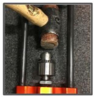
WHEN REFITTING THE CHUCK ENSURE THE TAPERED SPINDLE AND INTERNAL TAPER ON THE CHUCK ARE CLEAN FROM DEBRIS AND GREASE. (GIVE BOTH A VERY GOOD CLEAN BEFORE ASSEMBLY)
