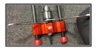
STEP 2=PLACE SPANNERS ON NUTS, HOLD THE 17MM SPANNER AND TURN THE 23mm SPANNER IN A ANTI-CLOCKWISE DIRECTION (THE NORMAL DIRECTION TO UNDO A NUT)
