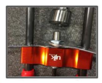
STEP 3=THE 24MM NUT WILL COME INTO CONTACT WITH THE CHUCK AND PRESS THE CHUCK OFF THE TAPERED SPINDLE.
