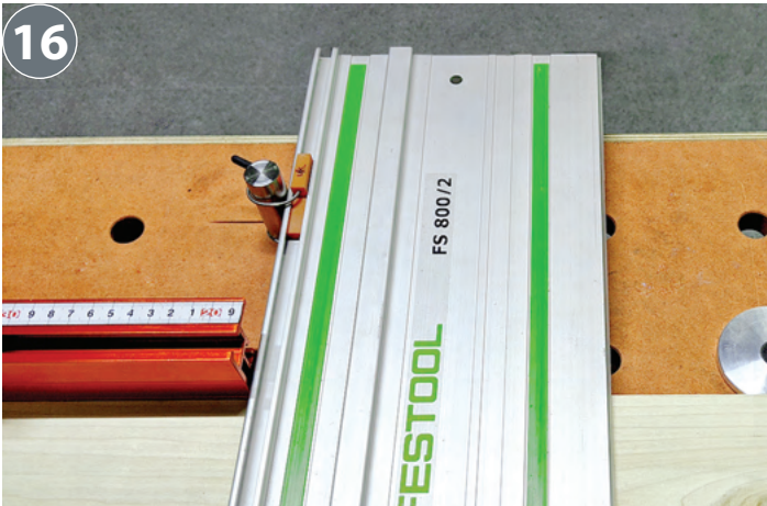
16-17. Refit your saw guide rail and you're ready to start cutting accurate lengths.
